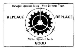
5. If the drive chain or sprockets are excessively worn or damaged, they should be replaced. Never use a new chain with worn sprockets; rapid chain wear will result.
