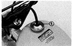
timing if knocking or pinging continues. After refueling, be sure to tighten the fuel tank cap firmly.
