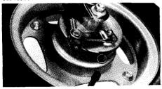
(2) Front brake adjusting nut
