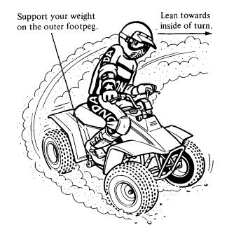
Incorrect turning techniques may cause the front wheels to slide straight ahead when steered without affecting the FOUR TRAX's direction of travel. If this should occur, close the throttle and come to a stop. Then continue practicing the technique outlined on the preceding page.
