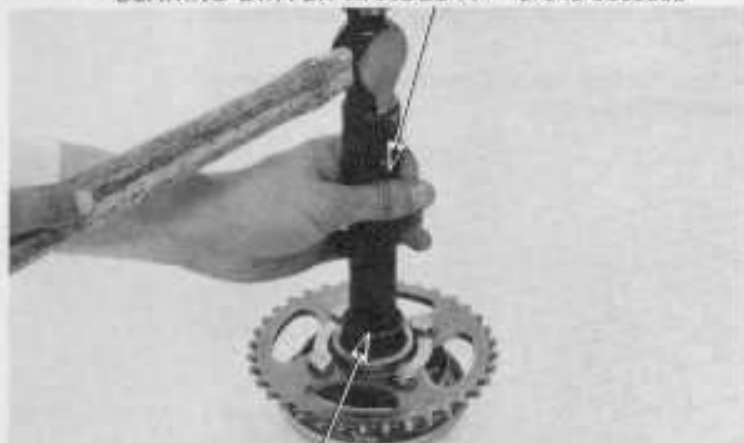
BEARING DRIVER OUTER, 37 x 40 mm — 07946-3000000 BEARING DRIVER PILOT, 17 mm
