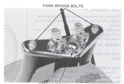
STEERING STEM NUT LOCK NUT WRENCH, 30 x 32 mm or 07716-0020400
