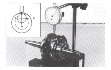
Spin the crankcase bearing by hand and check for play.
