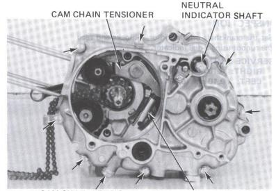
CAM CHAIN TENSIONER SEALING BOLT PUSH ROD
