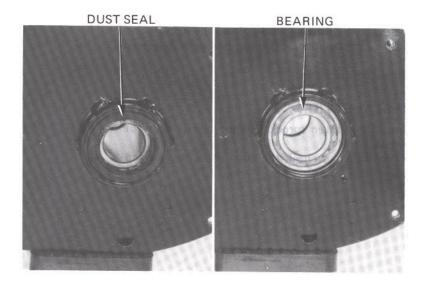
Pack all bearing cavities with grease. Drive in the new bearings.
