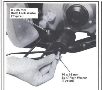
STEP 24—Install right and left step guards as shown using a 10 x 16 mm bolt/plain washer and an 8 x 25 mm bolt/lock washer for each. Tighten bolts to specified torque.
