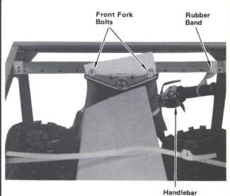
STEP 4—Loosen two front fork bolts. Remove rubber band holding handlebar to the crate frame.
