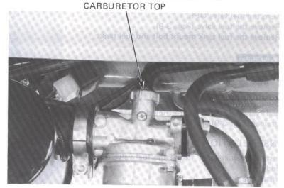
Turn the fuel valve OFF and remove the fuel valve by removing the two screws.
