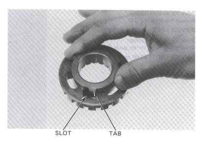
Install the primary drive gear and washer.
