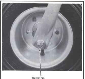
STEP 23—Insert cotter pin through slots in nut and hole in axle. Spread cotter pin ends as shown.
