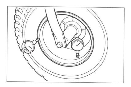
Set the axle in V-blocks, rotate and measure the runout with a dial indicator.
