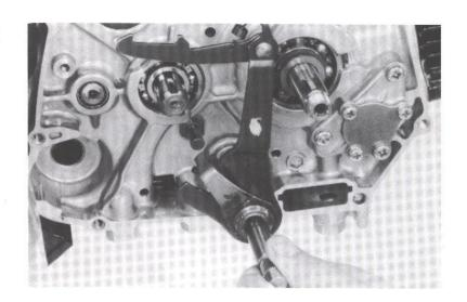
Install the pins onto the gearshift drum and install the washer and drum stopper plate as shown.
