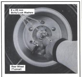
STEP 17—Inflate rear tires to 2.2 psi. Install rear wheels as shown using three 8 x 20 mm bolts/lock washers for each. Tighten bolts to specified torque.
