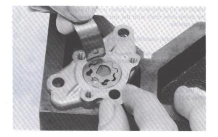
Place the oil pump cover gasket. Measure the rotor end clearance.
