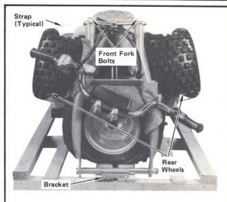
**STEP 6**—Cut strap holding rear wheels. Remove wheels. Retighten front fork bolts to specified torque.
