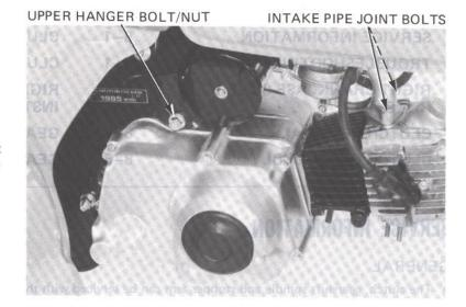
Remove the right crankcase cover bolts. Loosen the engine lower hanger bolt and lower the floor jack, then remove the right crankcase cover.
