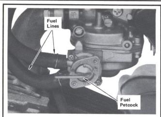
STEP 26-Inspect fuel tank. If necessary, drain and flush fuel tank by removing fuel lines. Reconnect fuel lines, fill tank, turn on fuel petcock and check for leaks. Drain residual fuel from carburetor.
