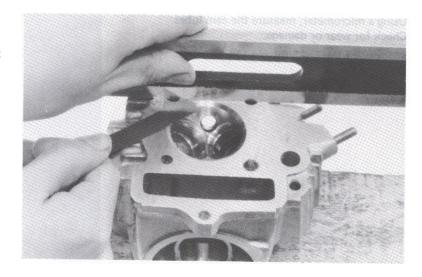
Inspect each valve for bending, burning, scratches or abnormal stem wear.
