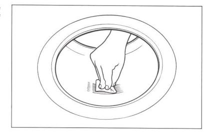
Apply rubber cement around the torn area and allow it to dry. Remove the lining from the patch and center it over the injury. Press the patch against the injury using a special roller.
