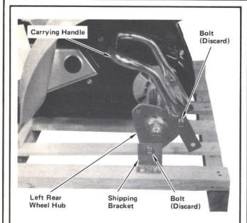
STEP 9—Remove bolt attaching carrying handle to wheel hub and remove carrying handle. Remove bolt attaching left rear wheel hub to shipping bracket. Discard bolts.
