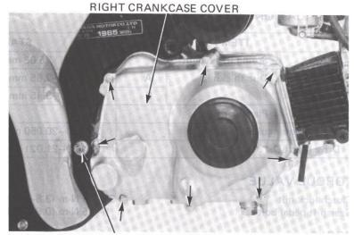
ENGINE LOWER HANGER BOLT/NUT
