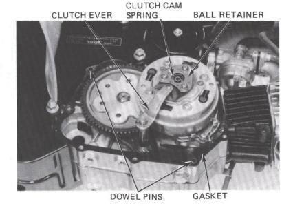
Install the clutch adjusting bolt and clutch lifter aligning the tang on the clutch lifter and groove on the right crankcase cover.
