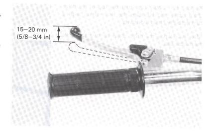
Adjust the brake lever free play by turning the adjuster nut.
