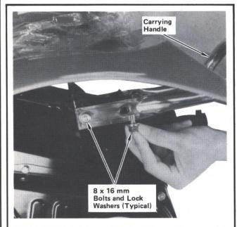
STEP 16—Install carrying handle on frame, with curved end up, using four 8 x 16 mm bolts and lock washers. Tighten bolts to specified torque.
