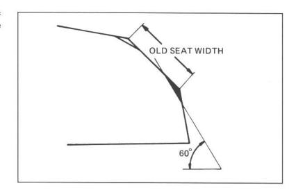
Install a 45 degree finish cutter and cut the seat to the proper width.
