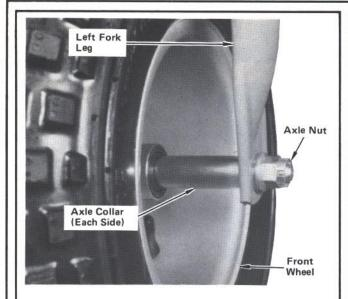
STEP 22—Position front wheel between fork legs with valve stem on left side. Insert axle from right side, through right fork leg, axle collar, wheel hub, axle collar, and left fork leg. Install axle nut and tighten nut to specified torque.
