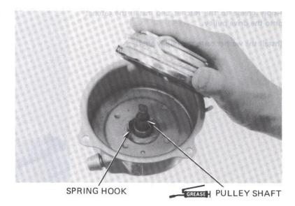
Preload the starter spring by turning the pulley 2 turns clockwise.
