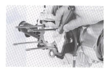
Install a new gasket, O-rings and dowel pins.
