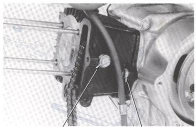
GUIDE ROLLER PIN CYLINDER MOUNT BOLT
