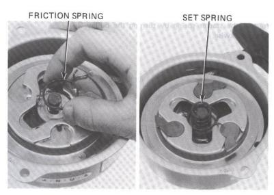
Install the ratchet cover and hook the friction spring into the ratchet cover.
