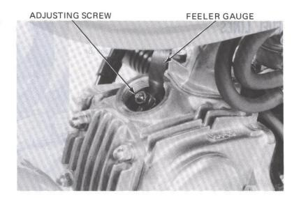
VALVE ADJUSTING WRENCH, 8 x 9 mm 07908—GE00200 or equivalent commercially available in U.S.A.
