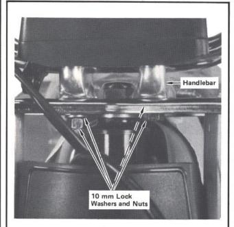
STEP 11—Install handlebar on upper fork bridge as shown using two 10 mm lock washers and nuts. Tighten nuts to specified torque.
