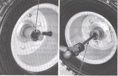
BEARING REMOVER SHAFT 07746—0050100 or Equivalent commercially available in U.S.A.
