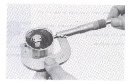
Measure the piston pin hole I.D.
