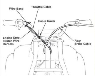
**STEP 15**—Check for proper routing of cables and wire harness as shown.
