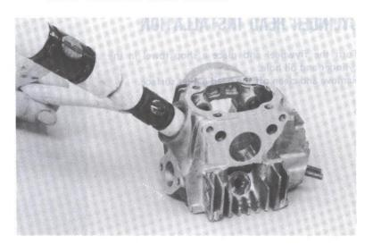
Install the camshaft with the camshaft hole facing down for easy camshaft sprocket installation.
