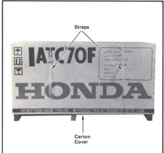
**STEP 1**—Cut straps and carefully lift off carton cover.
