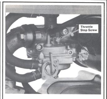
STEP 27-Adjust carburetor air screw, idle speed, and throttle free play as described in owner's manual or shop manual. Refer to owner's manual for use of speed limiter screw.
