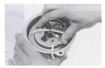
Route the rope end through the starter housing hole and install the handle.
