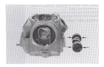
Measure the length of the inner and outer valve springs.
