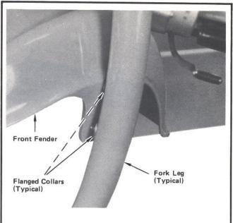
**STEP 19**—Position front fender between fork legs with short end forward. Position flanged collars between fork legs and front fender.
