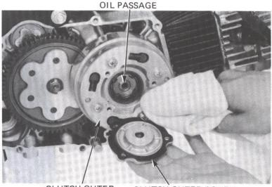
CLUTCH OUTER CLUTCH OUTER COVER
