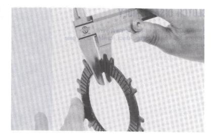
Check the rollers and plates for excessive wear or damage.
