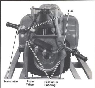
STEP 10—Remove ties holding handlebar to front fork legs. Remove protective padding from front forks. Remove front wheel from behind front forks.
