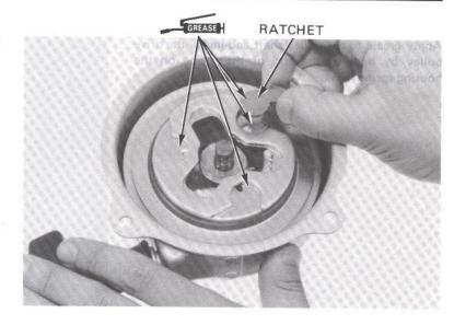
Install the friction spring as shown.
