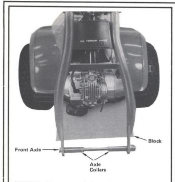
STEP 18—Remove and clean front axle and axle collars. Place a padded block under engine to raise front forks.
