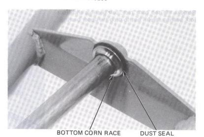
Install a new washer and dust seal and drive a new cone race into place.
