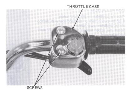
Remove the handlebar upper holder cover cap and remove the two screws, then remove the handlebar upper holder cover.
