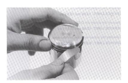
Insert each piston ring into the cylinder, and measure the end gap.
