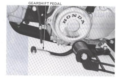
Remove the right crankcase cover (Page 8-2). Remove the drum stopper arm, Remove the drum stopper plate and washer.
