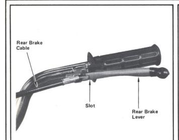
STEP 14—Route rear brake cable in front of throttle cable and insert end of rear brake cable into slot in brake lever. Pull cable back through slot in brake lever bracket.
