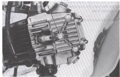
Hold the flywheel and remove the three attaching bolts and the cam sprocket.
