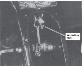
STEP 28-Place a block under ATC. Spin rear wheels by hand and measure free play of rear brake lever before brake starts to engage. Free play, measured at tip of rear brake lever, should be between 25-30 mm (1-1½ in.). Use adjusting nut on brake operating rod at rear of ATC to make adjustment. Remove block from under ATC.
