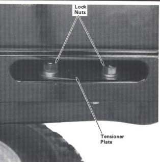
STEP 29—Remove drive chain inspection hole cover and check for a drive chain slack of 10-20 mm (3/8-3/4 in.). If necessary, adjust drive chain slack as follows. Stop engine and position vehicle to obtain access to chain tensioner plate through hole in skid plate. Loosen the two lock nuts and move tensioner plate to obtain correct chain slack. Tighten bolt lock nuts securely. Reinstall inspection hole cover.
