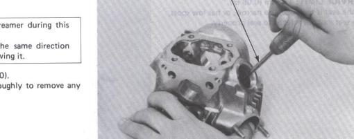
Ream the new valve guide after installation.
