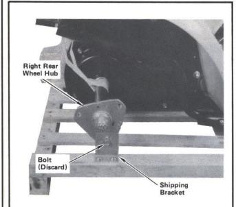
**STEP 7**—Remove bolt attaching right rear wheel hub to shipping bracket. Discard bolt.
