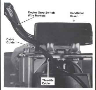
STEP 12—Route engine stop switch wire harness and throttle cable down through cable guide as shown. Tighten screw securely and push cable guide up to edge of handlebar cover.
