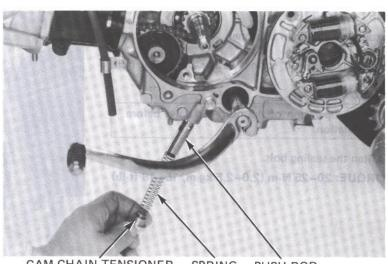
CAM CHAIN TENSIONER SPRING PUSH ROD SEALING BOLT
