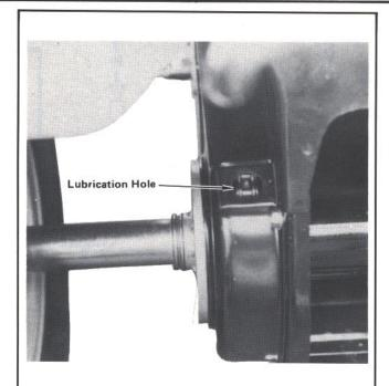
**STEP 30**—Remove lubrication hole cover and lubricate drive chain using a commercially prepared chain lubricant. Reinstall hole cover.
