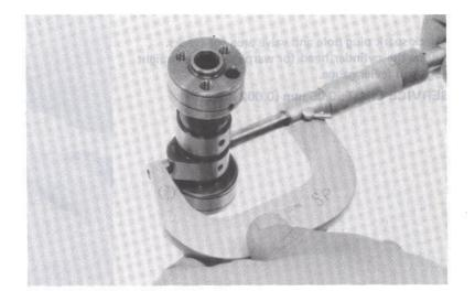
Measure and record the camshaft journal O.D. Measure and record the camshaft bearing I.D. in the cylinder head.
