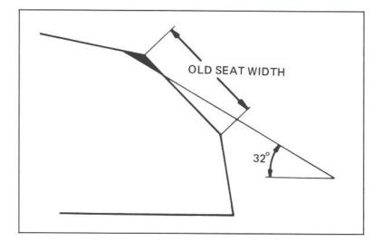
Use a 60 degree cutter to remove the lower 1/4 of the old seat. Remove the cutter and inspect the area you have just cut.
