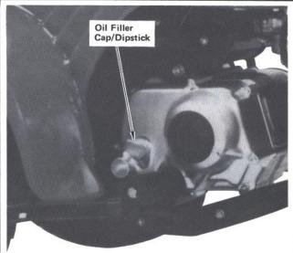
STEP 25—Remove oil filler cap/dipstick. Check engine oil level and if necessary add recommended oil as described in owner's manual or shop manual. Reinstall oil filler cap/dipstick.
