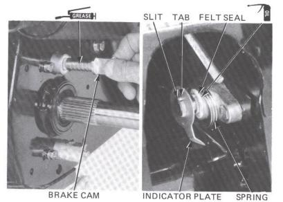
Install the brake arm over the brake arm aligning the punch mark on the brake arm with the slit on the brake cam.
